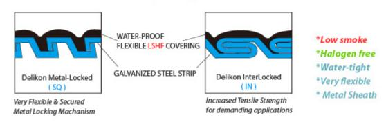
Low Smoke Zero Halogen Jacketed Flexible Metal Conduit LSZH, LSOH, LSOH, LSFH, OHLS
